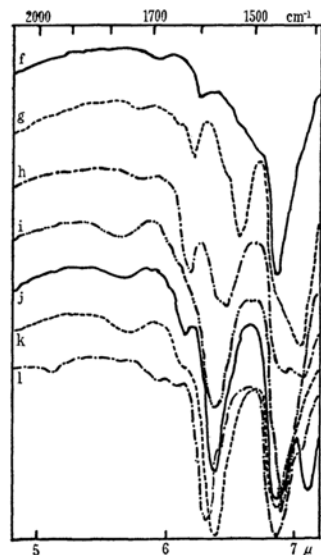
Fig. 4. Infrared absorption spectra of: (f), \text{H}[\text{Co}(\text{dgH})_2\text{Br}_2] ; (g), \text{H}[\text{Co}(\text{dgH})_2(\text{NO}_2)_2] ; (h), \text{Na}[\text{Co}(\text{dgH})_2(\text{NO}_2)_2] ; (i), [\text{Co}(\text{OH}_2)(\text{dgH})_2(\text{NO}_2)] ; (j), [\text{Co}(\text{NH}_3)(\text{dgH})_2(\text{NO}_2)] ; (k), [\text{Co}(\text{NH}_3)(\text{dgH})_2\text{Cl}] ; (l), [\text{Co}(\text{NH}_3)_2(\text{dgH})_2\text{Cl}] .
